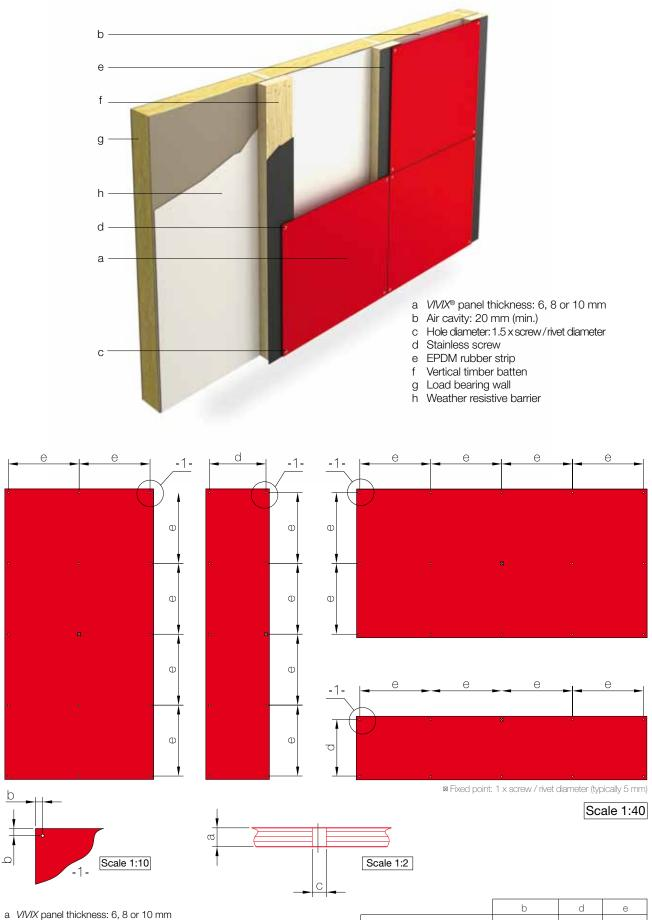
b Typical edge distance: min 20 mm - max see table on right
